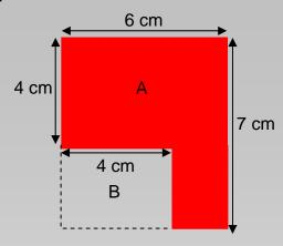
You can also calculate the area of this shape by calculating the area of the large rectangle (A) and subtracting the area of the small rectangle (B).
