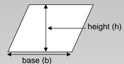
Area of a parallelogram = base × height
